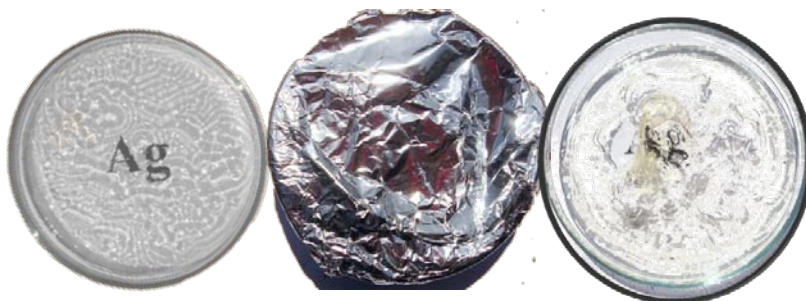
Fig. S12. I) Polymerized acrylamide gel along with Ag(I)SG. II) Sample covered with aluminium foil and exposed to sunlight in outdoor air. III) No visible color change after 6 h of exposure to sunlight. The ambience was at 35°C.
