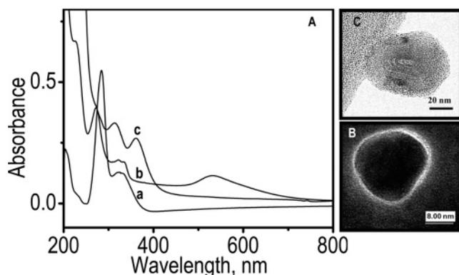
**Figure 1.** (A) UV-vis spectrum of (a) free ciprofloxacin, (b) Au@ciprofloxacin@SiO<sub>2</sub>, and (c) cip@SiO<sub>2</sub>. (B) shows an image of a Au@SiO<sub>2</sub> core-shell nanoparticle taken with an energy loss of 15 eV, and (C) shows the TEM image of the carbon onion structure formed inside the silica shell.
