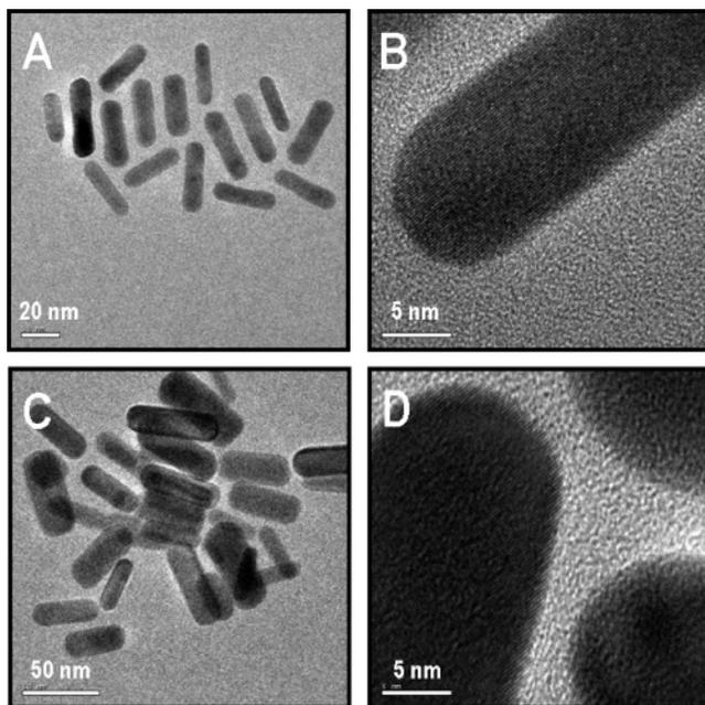
**Figure 4.** HRTEM images of neat AuNR (A, B) and AuNR@Mb (C, D). Panels B and D are lattice resolved.
