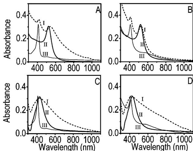
**Figure 1.** Absorption spectra of the M@X nanoparticle system. The panels A, B, C, and D correspond to the samples Au@Mb, Au@Hb, Ag@Mb, and Ag@Hb, respectively. Traces I, II, and III of all figures correspond to 0.2 mg/mL M@X, 0.1 mg/mL M@Cit, and 0.1 mg/mL X, respectively.
