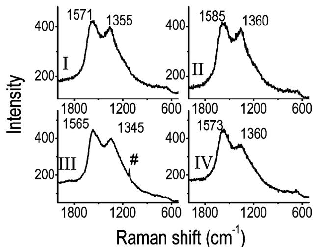
**Figure 5.** Raman spectra recorded using 514.5 nm laser excitation through a confocal (60 X) objective. The traces I, II, III, and IV correspond to Mb, Ag@Mb, Hb, and Ag@Hb, respectively. The peak around 1100 cm<sup>-1</sup> (marked with #) in trace III corresponds to the Raman feature of the cover glass slip used for the experiment.
