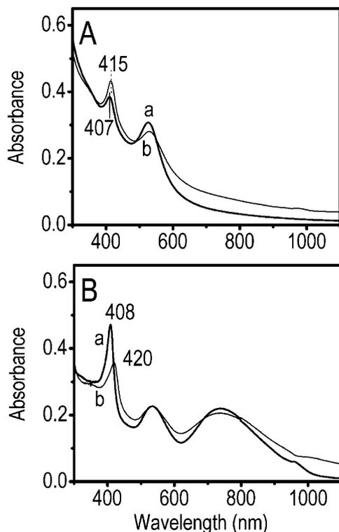
**Figure 7.** UV-visible spectrum of the samples in aqueous phosphate buffered saline (PBS). (A) Au@Hb (thick trace, a) and Au@Hb-N<sub>3</sub> (thin trace, b); (B) AuNR@Mb (thick trace, a) and AuNR@Mb-N<sub>3</sub> (thin trace, b).
