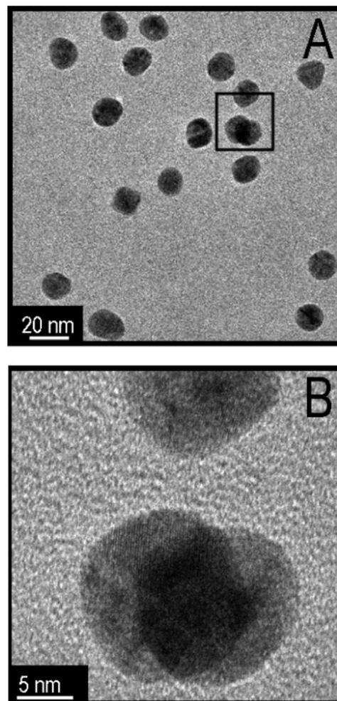
**Figure 8.** TEM images of Au@Hb-N<sub>3</sub>. Well-separated particles are observed in image A. The image B corresponds to an enlarged view of the marked portion in image A, showing the lattices of the gold nanoparticles.
