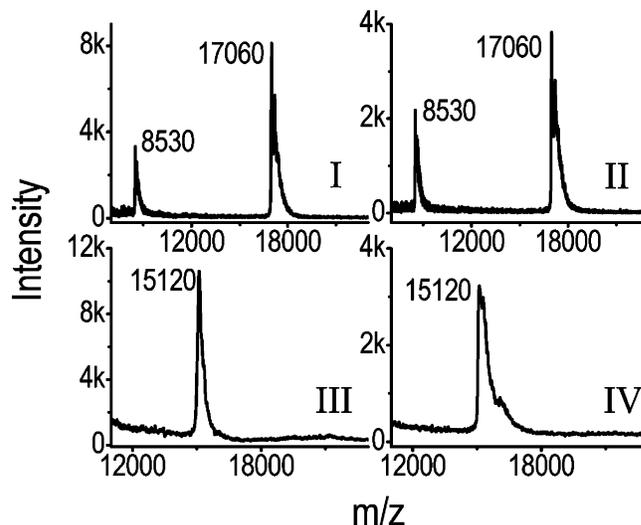
**Figure 6.** MALDI-TOF mass spectra of the samples measured with 337 nm N<sub>2</sub> laser using sinapinic acid matrix. The traces I, II, III, and IV correspond to Mb, Au@Mb, Hb, and Au@Hb, respectively.
