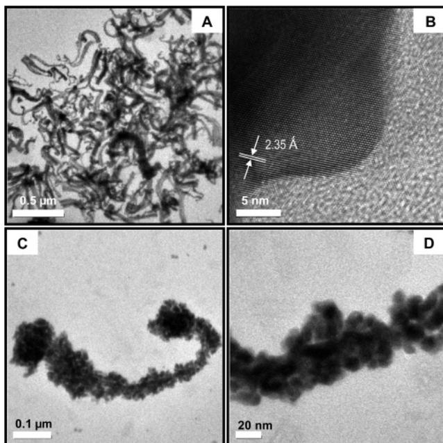
**Figure 3.** TEM images of gold nanowires at various magnifications formed when 10  $\mu\text{L}$  aniline was used. (B) The lattice resolved image of a part of the nanowire. (C) The TEM image of a single nanowire. (D) An enlarged portion of (C).
