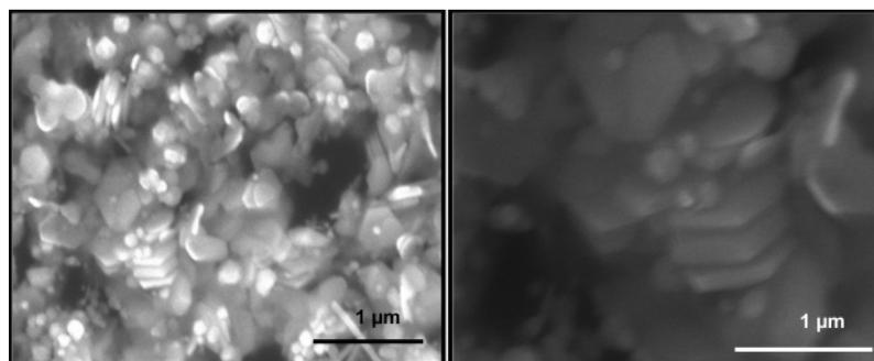
**Figure 4.** SEM images of the gold nanoplates formed when the reaction was carried out using the oligoaniline AuNPs synthesized by using 250  $\mu\text{L}$  of aniline.
