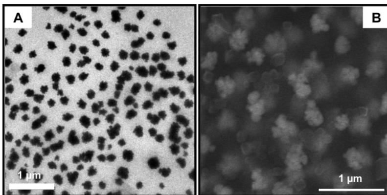
**Figure 5.** TEM (A) and SEM (B) images of the flower-like nanoparticles formed in the presence of KI.
