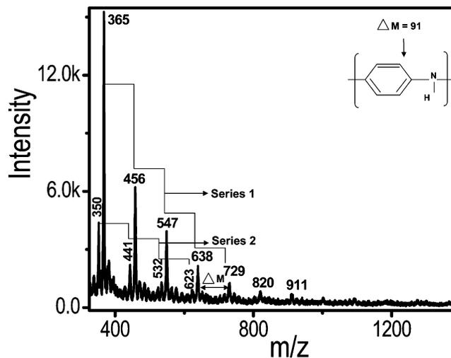
**Figure 9.** LDI mass spectrum of the PANI-coated gold nanowire taken in the linear positive mode.
