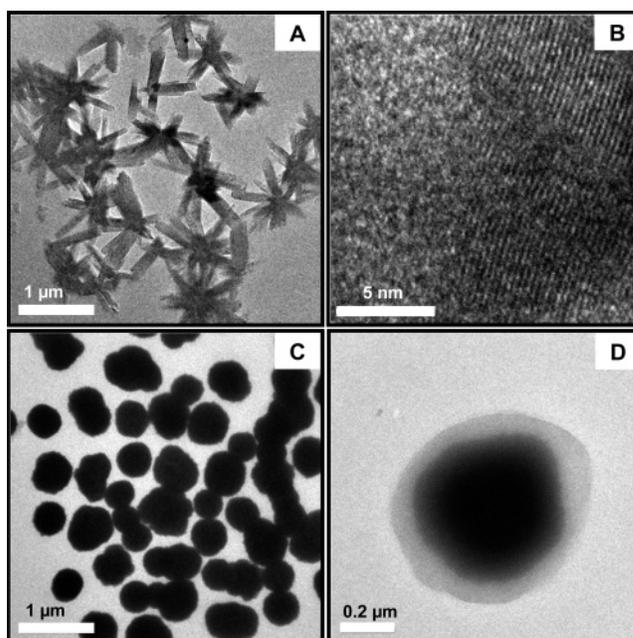
**Figure 7.** (A) TEM image of the nanowires at pH 2.5. (B) The lattice-resolved image of a region in A. (C) The TEM image of the nanowire at pH 10.2. (D) TEM image of the nanowire after the reversal of the pH from 10.2 to 2.9.
