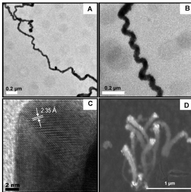
**Figure 2.** TEM images of gold nanowires at various magnifications when  $100 \mu\text{L}$  aniline was used. (C) The lattice resolved image of one part of the nanowire. (D) The SEM image of the gold nanowire synthesized in the same condition.
