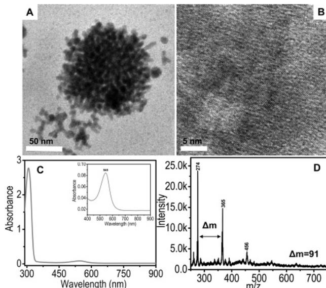
**Figure 1.** (A) TEM image of a single oligomeric-aniline-coated AuNP aggregate. (B) A lattice-resolved TEM image taken from the same nanoparticle. (C) UV-vis spectrum of oligomeric aniline-coated AuNPs. (D) LDI MS of oligoaniline-coated AuNPs. Inset of panel C shows an enlarged portion of the absorption spectrum.
