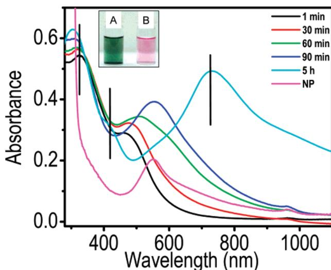
**Figure 6.** Time-dependent UV-vis spectra showing the formation of PANI-coated gold nanowires. The absorptions of PANI are marked. Inset shows the photographs of (A) the PANI-coated nanowire and (B) the precursor nanoparticle solution.
