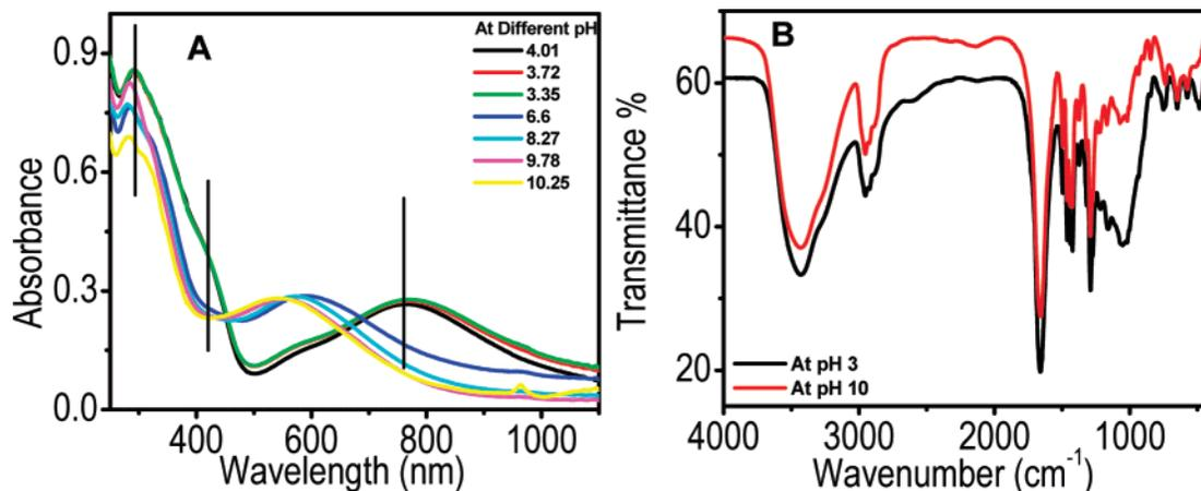
**Figure 8.** (A) The UV-vis spectra of the Au/PANI nanowire samples at different pH values, and (B) the IR spectra of the same sample at different pH values.
