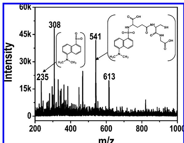
**Figure 2.** Positive-ion ESI-MS of the reaction product showing the features of dansyl glutathione ( $m/z$  541), glutathione ( $m/z$  308), dansyl group ( $m/z$  235), and glutathione dimer ( $m/z$  613). Molecular mass of dansyl glutathione is 540, and that of the dansyl fragment is 234 (the fragments are shown in the figure). ESI-MS (water:methanol 1:1, 20 ppm sample) shows the protonated ions. These features were seen in the exchange product also.
