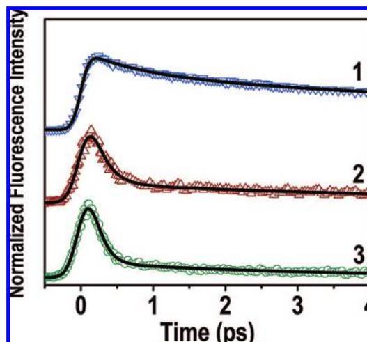
**Figure 6.** Femtosecond time-resolved fluorescence transients of (1) D-GSH, (2) reaction, and (3) exchange products. The samples were excited at 364 nm, and the transients were collected at 500 nm.
