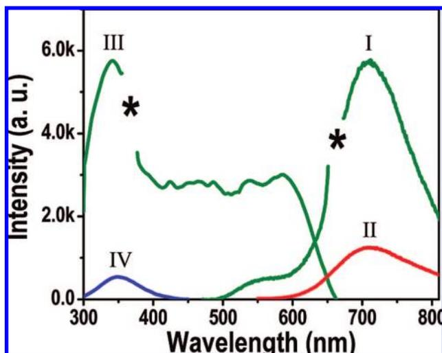
**Figure 5.** Steady-state fluorescence spectra of the reaction product. (I and II) Emission spectra obtained when excited at 330 and 535 nm, respectively, showing the same emission maximum. (III and IV) Corresponding excitation spectra for emission at 700 and 550 nm. The emission at 550 nm is the quenched donor emission. Asterisks correspond to regions where higher order lines of the grating mask the spectrum.
