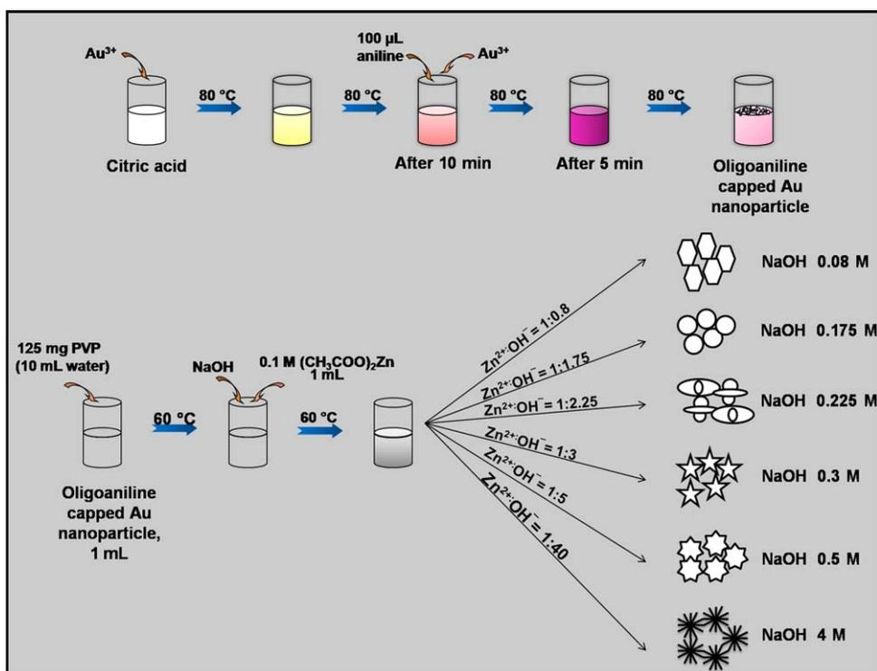
Scheme 1. Procedure used for the synthesis of various anisotropic zinc oxide nanostructures using Au/PANI.
