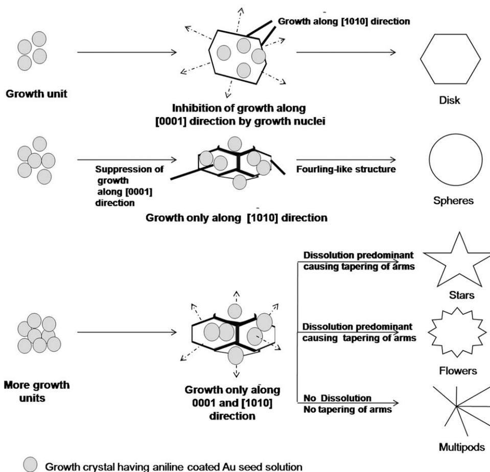
Fig. 8. Schematic representation of the growth of various ZnO nanostructures using Au-oligoaniline seeds.
