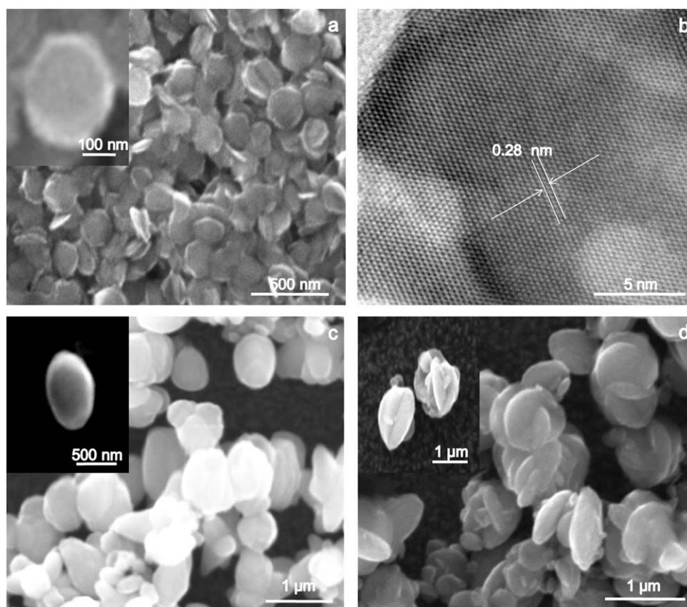
**Fig. 1.** (a) Large area SEM image of hexagonal plates. Enlarged SEM image of a hexagonal plate is in the inset; (b) high-resolution TEM image of the tip of a hexagonal plate; (c) large-area SEM image of the spheres. SEM image of a sphere is shown as inset; and (d) large-area SEM images of branched plates obtained at higher concentration of NaOH. Inset shows the small-area SEM image of these structures.
