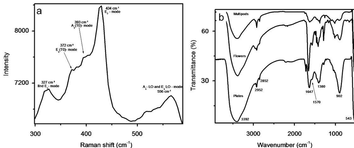
Fig. 6. (a) Raman spectra of the star-shaped zinc oxide structure synthesized using Au oligoaniline. The Raman spectra of different structures showed similar features; (b) FT-IR spectrum of hexagonal plates, flower and multipods shown from bottom to top, respectively.
