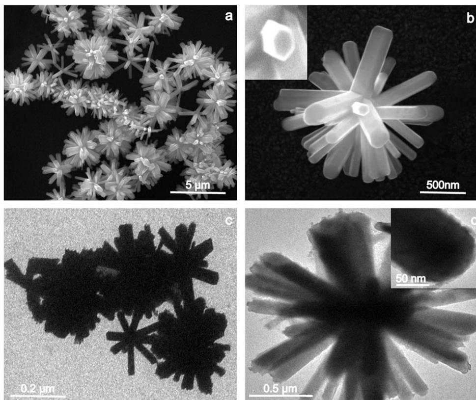
**Fig. 4.** (a) Large-area SEM image of the multipods; (b) SEM image of a single multipod; (c) and (d) large-area and small-area TEM images, respectively, of the multipods. TEM image of a tip is shown in the inset of d.
