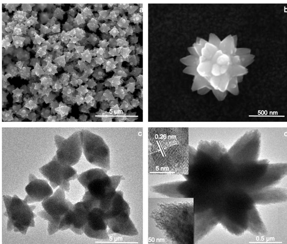
**Fig. 3.** (a) Large-area SEM image of the microflowers; (b) SEM image of a single flower; (c) and (d) large-area and small-area TEM images of the microflowers. TEM image of the tip and its corresponding HRTEM are inserted as the bottom and top insets, respectively.
