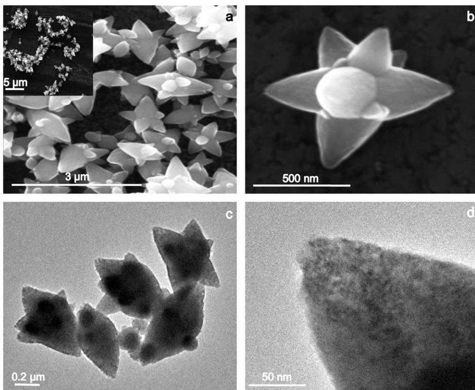
**Fig. 2.** (a) Large area SEM image of the star structure. The clinging tendency of these structures is shown in the inset; (b) SEM image of a single star; (c) large area TEM image of the star structure; and (d) TEM image of a single tip.
