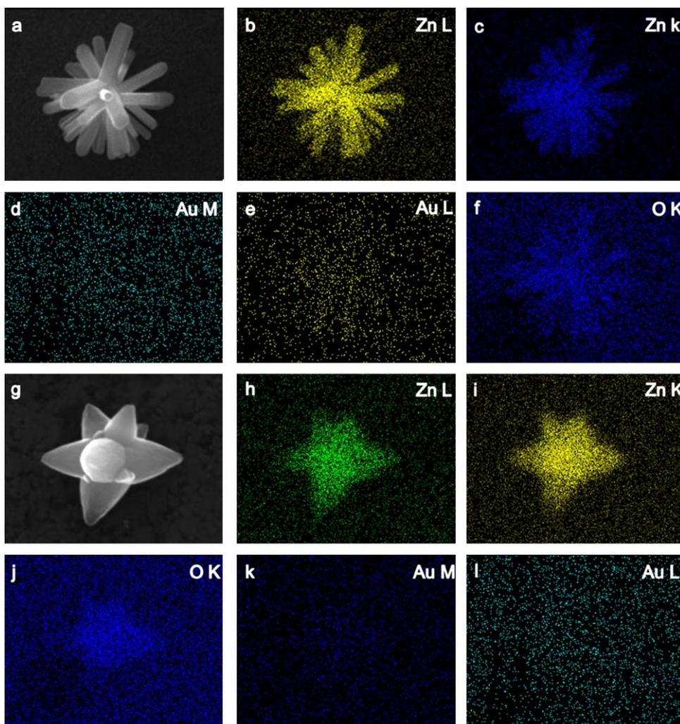
Fig. 5. Insets b–f and h–l shows the EDAX spectra of multipods and stars, respectively. The SEM images of both these structures are shown in a and g.
