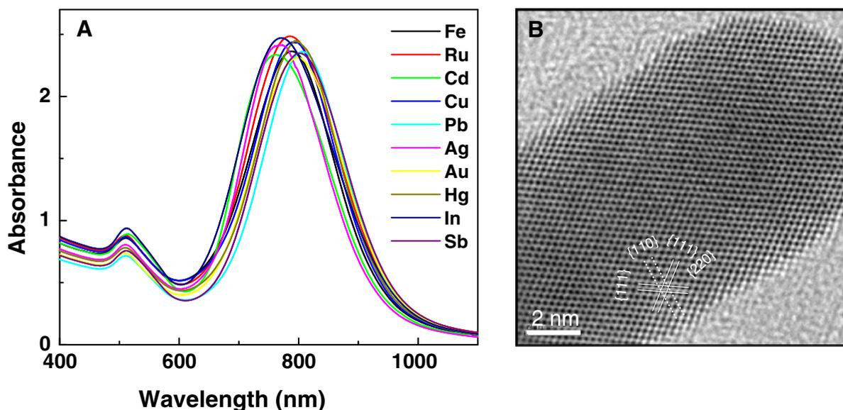
**Fig. 2** **A** UV–visible spectra of GNRs formed using various metal seeds. **B** HRTEM of one end of a GNR formed from Pb seeds showing its fcc crystal structure
