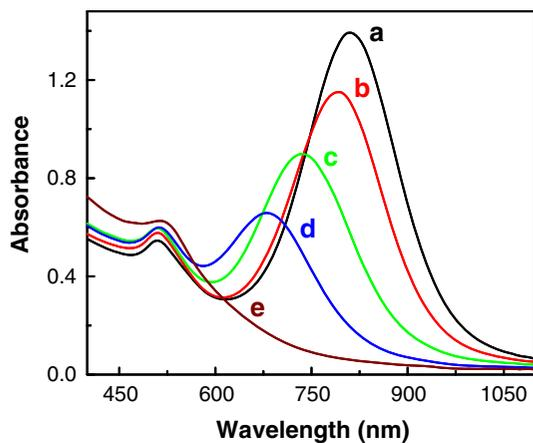
**Fig. 5** UV-visible spectra of GNRs formed with increasing amount of  $\text{NaBH}_4$ : a 50  $\mu\text{L}$ , b 100  $\mu\text{L}$ , c 200  $\mu\text{L}$ , d 300  $\mu\text{L}$ , and e 500  $\mu\text{L}$
