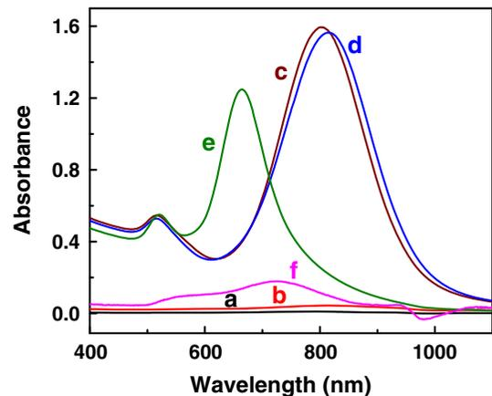
**Fig. 7** Absorption spectra of GNRs synthesized with a aged NaBH<sub>4</sub>, b heated and cooled NaBH<sub>4</sub>, c freshly prepared NaBH<sub>4</sub>, d fresh Au seed, e Au seed at 1 h, and f 4 h after preparation
