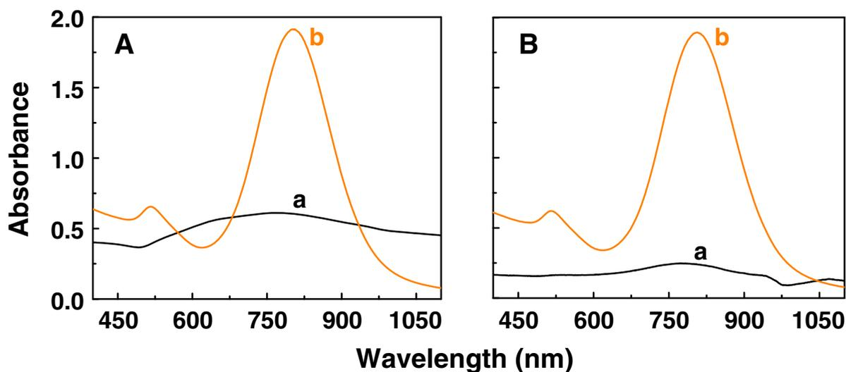
**Fig. 8** UV-visible spectra of GNRs prepared by using (A) *a* 50  $\mu\text{L}$  of aged  $\text{NaBH}_4$  (kept for more than 8 h at room temperature) and *b* freshly prepared 50  $\mu\text{L}$   $\text{NaBH}_4$  added to
