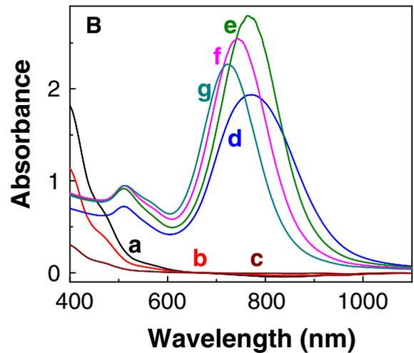
**Fig. 6** UV–visible spectra of GNRs prepared using different amount of **A** Au<sup>3+</sup> ions [a 50 μL, b 100 μL, c 200 μL, d 250 μL, e 300 μL, f 400 μL, g 500 μL, and h when 35 μL more AA was added to existing (g) solution], and **B** AA [a
