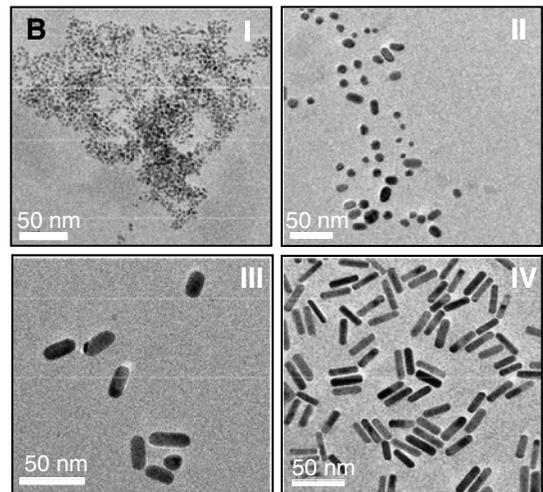
**Fig. 4** **A** UV–visible spectra of GNRs obtained at different time intervals after adding  $\text{NaBH}_4$  solution: *a* 0, *b* 3, *c* 5, *d* 8, and *e* 10 min. **B** TEM images of nanorods formed at different stages after adding  $\text{NaBH}_4$  solution: (I) 3, (II) 5, (III) 8, and
