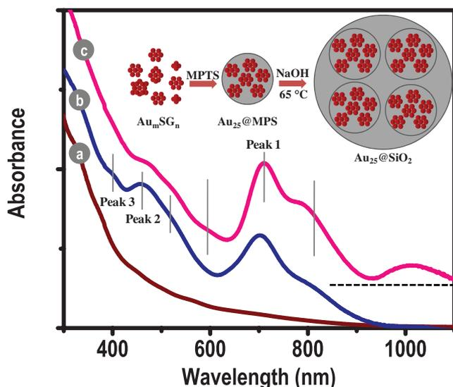
**Figure 1.** Optical absorption spectra of a)  $Au_mSG_n$ , b)  $Au_{25}@MPS$ , and c)  $Au_{25}@SiO_2$ . The features of the QCs are indicated with lines (see the text for explanation).
