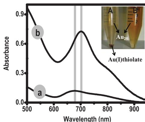
**Figure 4.** Comparison of the absorbance of *peak 1* of  $\text{Au}_{25}$  formed by a) GSH- and b) MPTS-mediated syntheses. Inset shows photographs of the reaction products upon reaction with A) GSH and B) MPTS, after centrifugation.
