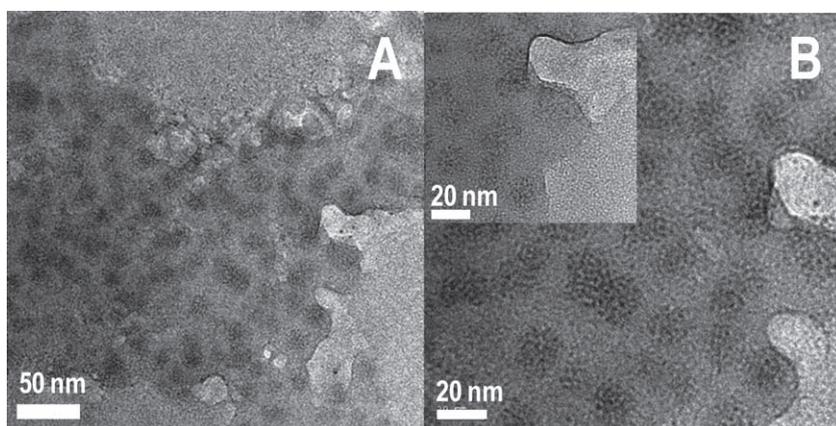
**Figure 3.** A) Low- and B) high-magnification TEM images of  $\text{Au}_{25}@SiO_2$ . A portion of (B) is expanded in the inset.
