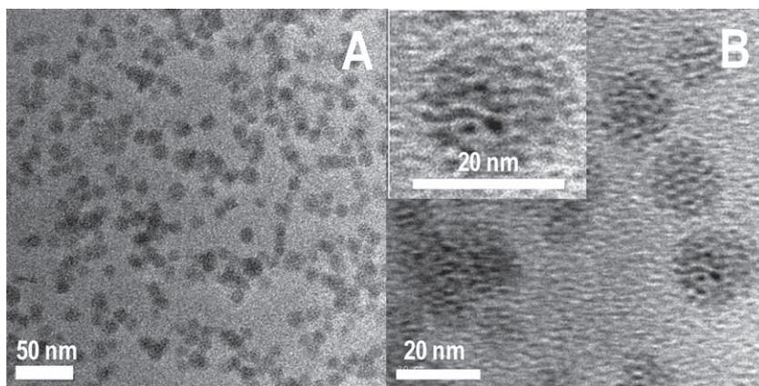
**Figure 2.** A) Low- and B) high-magnification TEM images of  $Au_{25}@MPS$ . A portion of (B) is expanded in the inset.
