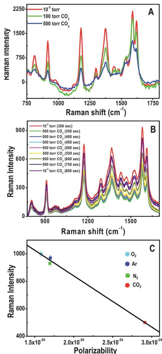
**Fig. 3** (A) SERS spectrum collected at different concentrations of CO<sub>2</sub>. (B) Change in SERS intensity of Au@MSA SL crystals under 500 Torr of CO<sub>2</sub> at different time intervals. (C) Change in Raman intensity vs. polarizability of gases at 500 Torr (O<sub>2</sub>, Ar, N<sub>2</sub> and CO<sub>2</sub>).
