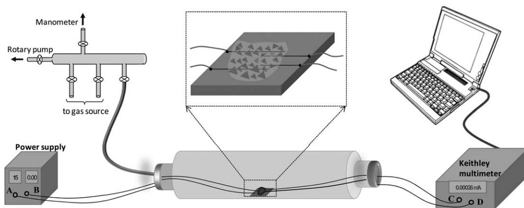
**Scheme 1** Representation of the set-up used for measuring  $I$ - $V$  characteristics of SLs. Triangles shown are SLs.
