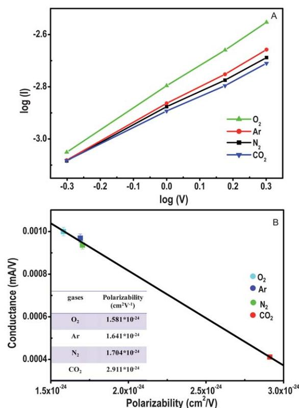
**Fig. 2** (A) Plot of log current (mA) vs. log voltage (V) of the SL crystals upon exposure to gases,  $\text{O}_2$ , Ar,  $\text{N}_2$ , and  $\text{CO}_2$  at 500 torr. (B) Conductance (slope of  $I$  vs.  $V$ , in  $\text{mA V}^{-1}$ ) vs. polarizability ( $\text{cm}^2 \text{V}^{-1}$ ) of the corresponding gases. Table in the inset shows the polarizability of all the four gases under consideration.
