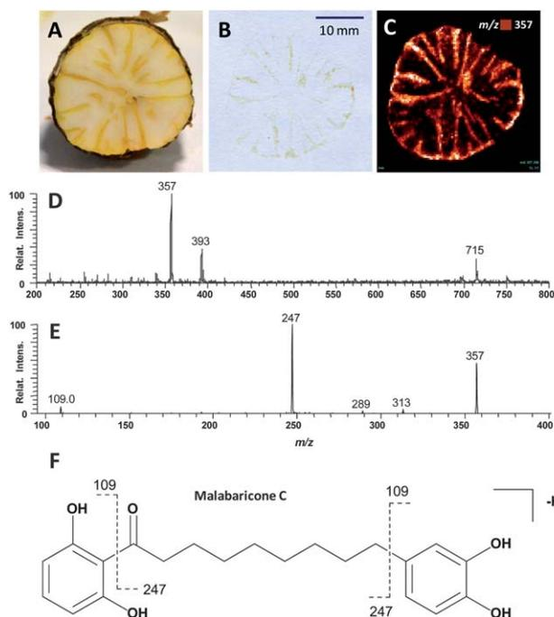
**Fig. 1** (A) Cross-sectional view of a *Myristica malabarica* seed. (B) Blot onto printer paper. (C) Chemical image showing the distribution of  $m/z$  357 species, deprotonated malabaricone C. (D) Average mass spectrum in negative ion mode of one line scan across the surface. (E) Tandem mass spectrum of  $m/z$  357, deprotonated malabaricone C. (F) Structure of malabaricone C. Scale bar (10 mm) applies to all figures.
