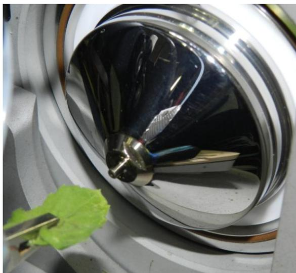
**Figure S2.** Experimental set-up for the leaf spray ionization showing the Tulsi leaf connected with a clip and held in front of atmospheric inlet of the mass spectrometer.
