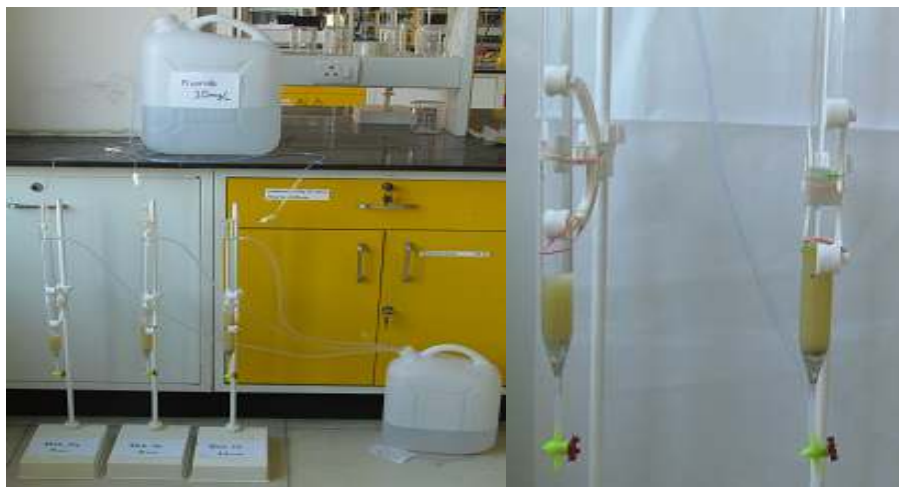
Figure S1: photographs showing the continuous column experiment set up. The granules sizes of the SANA used in the study are in the range of 0.3 to 1.18 mm.
