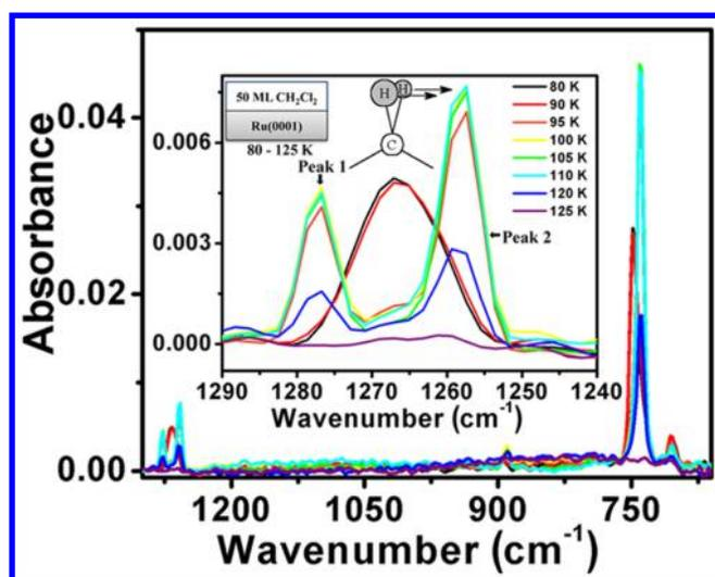
**Figure 1.** Temperature-dependent RAIR spectra of 50 ML  $\text{CH}_2\text{Cl}_2$  deposited at 80 K on Ru(0001). Inset shows the expanded view of the  $-\text{CH}_2$  wagging region and schematic of the surface under investigation.
