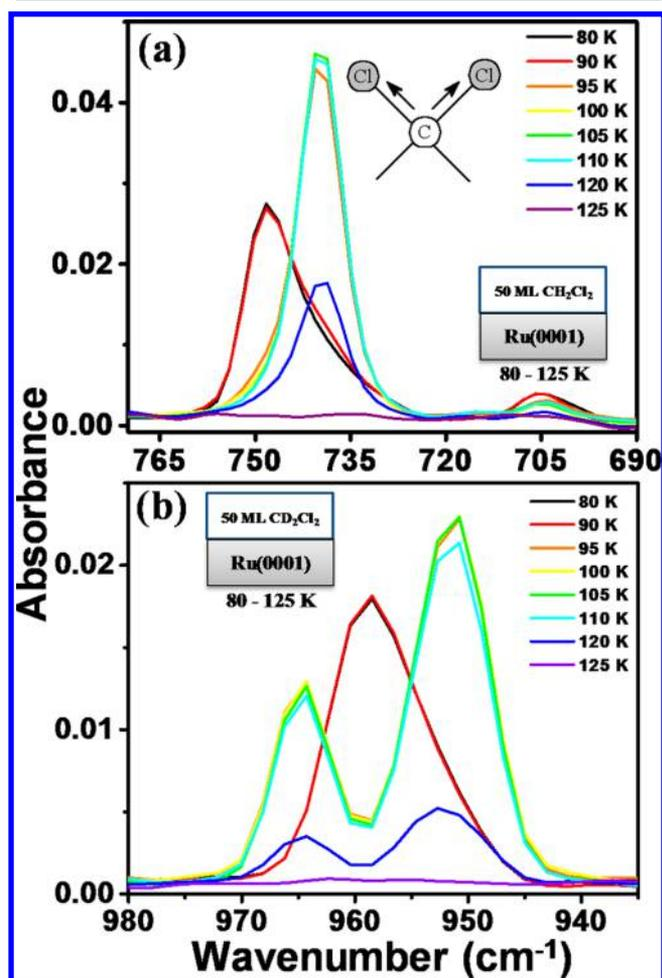
**Figure 2.** Temperature-dependent RAIRS study on a molecule to find changes in vibrational spectra upon heating. Spectra corresponding to (a) C–Cl antisymmetric stretching ( $\text{CH}_2\text{Cl}_2$ ) mode and (b)  $-\text{CD}_2$  wagging modes ( $\text{CD}_2\text{Cl}_2$ ) are compared when 50 ML of  $\text{CX}_2\text{Cl}_2$  ( $X = \text{H}$  or  $\text{D}$ ) is deposited on Ru(0001) at 80 K and warmed. Insets show the schematic of the surfaces during experiment.
