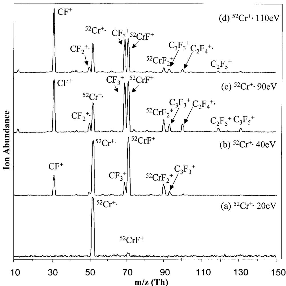
**Figure 1.** Scattered ion mass spectra recorded upon collision of  $^{52}\text{Cr}^+$  at a fluorocarbon monolayer surface at various incident energies. The collision energies and the ion/surface reaction products are indicated.
