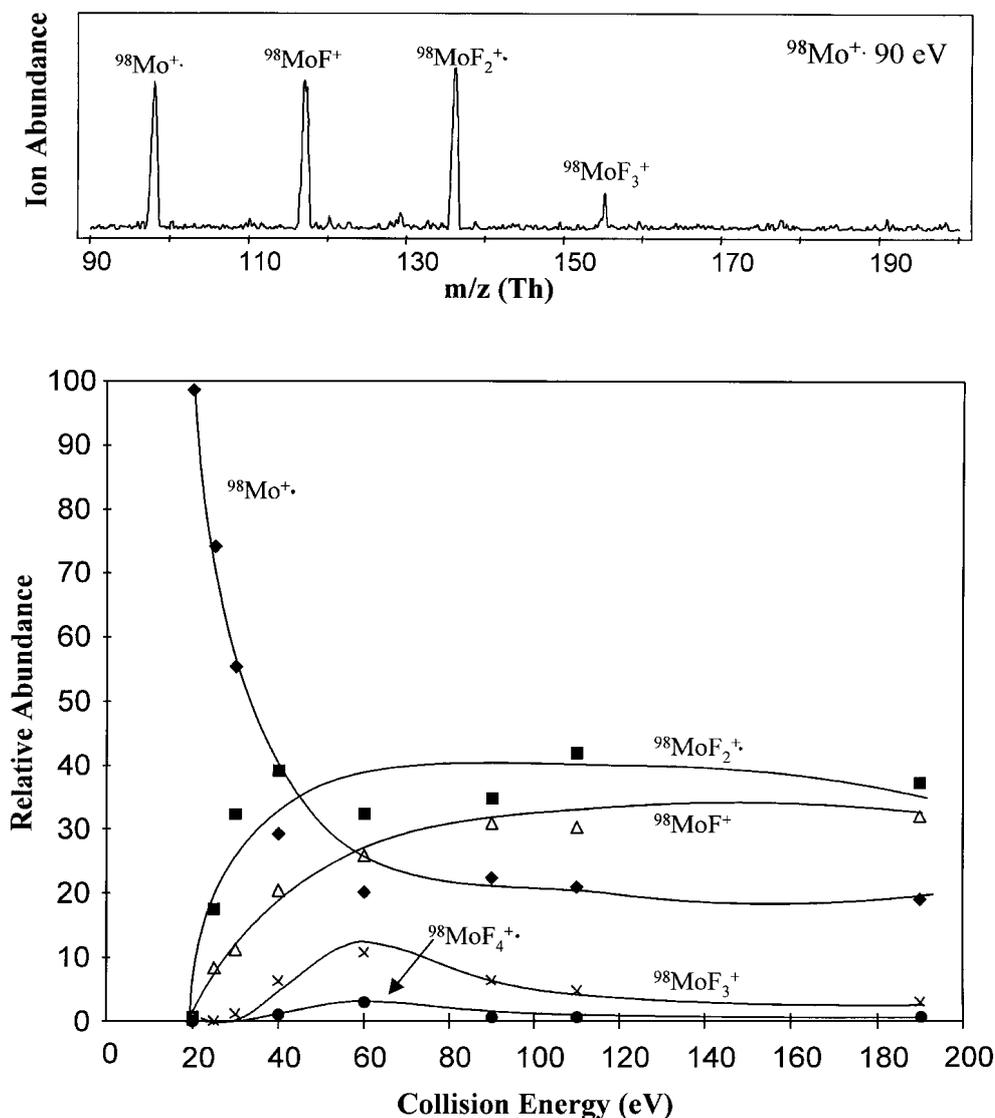
**Figure 2.** The top panel displays the scattered ion mass spectra (90 Th and above) at 90 eV. The bottom panel displays an energy resolved mass spectrum (ERMS) plot for the ion/surface reaction products produced upon collision of  $^{98}\text{Mo}^{+\cdot}$  at a fluorocarbon monolayer surface in a collision energy range from 20 to 200 eV.
