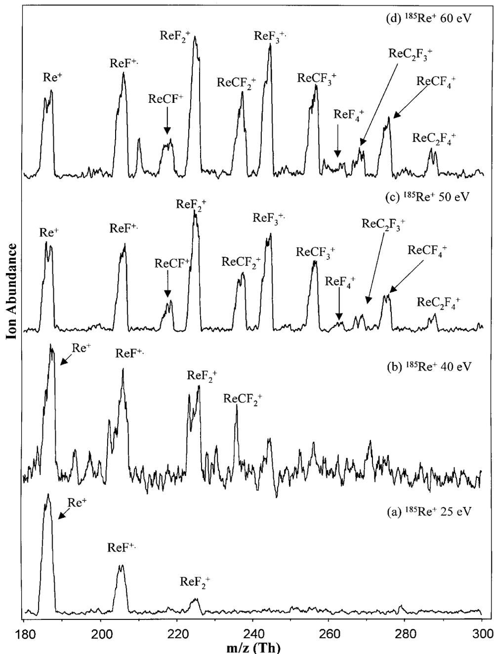
**Figure 4.** Scattered ion mass spectra (180 Th and above) recorded upon collision of  $^{187}\text{Re}^+$  at a fluorocarbon monolayer surface at various incident energies. Due to low primary ion current, the 35 eV spectrum is noisy. The collision energies and the ion/surface reaction products are indicated.
