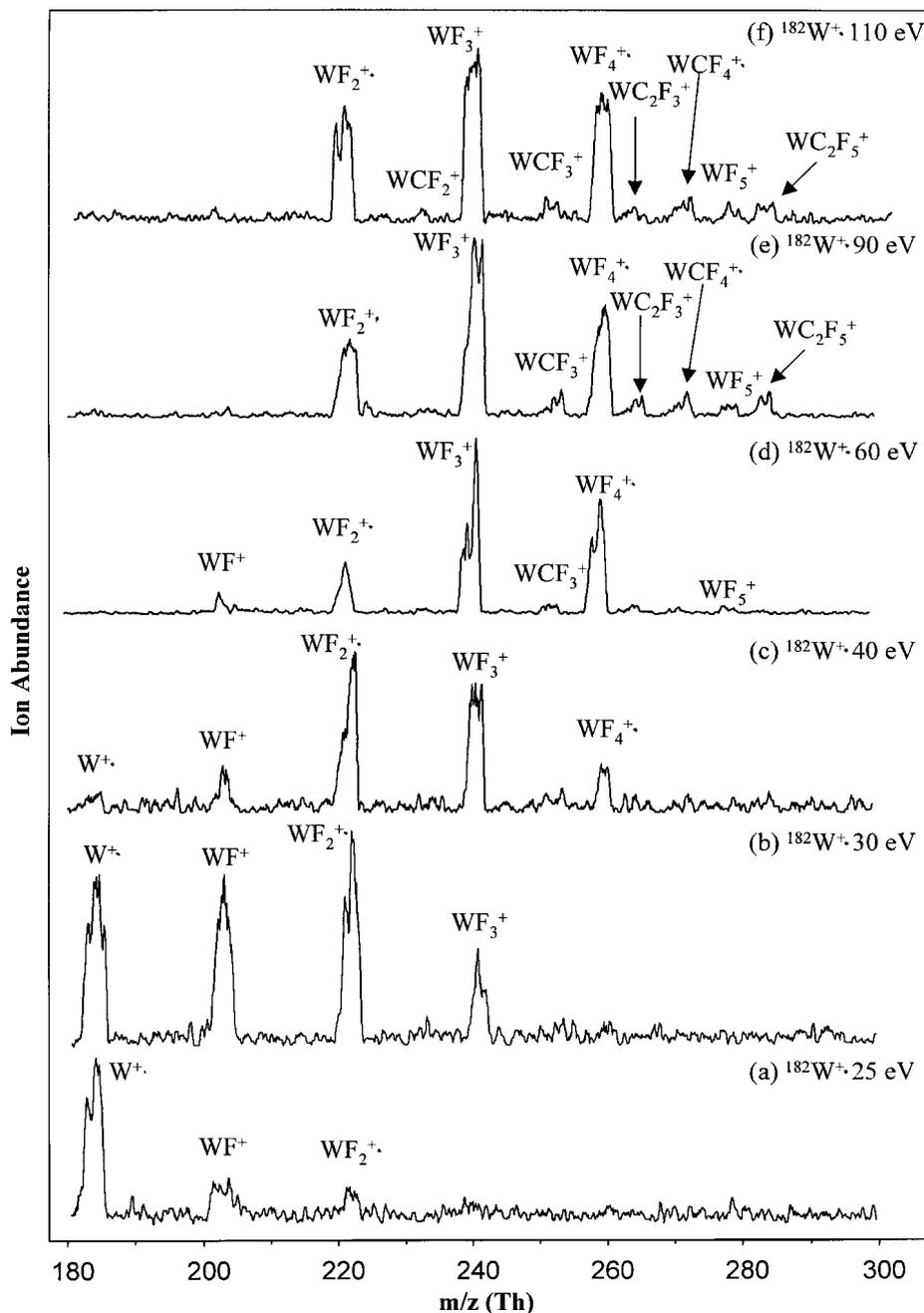
**Figure 3.** Scattered ion mass spectra (180 Th and above) recorded upon collision of  $^{182}\text{W}^+$  at a fluorocarbon monolayer surface at various incident energies. The collision energies and the ion/surface reaction products are indicated.
