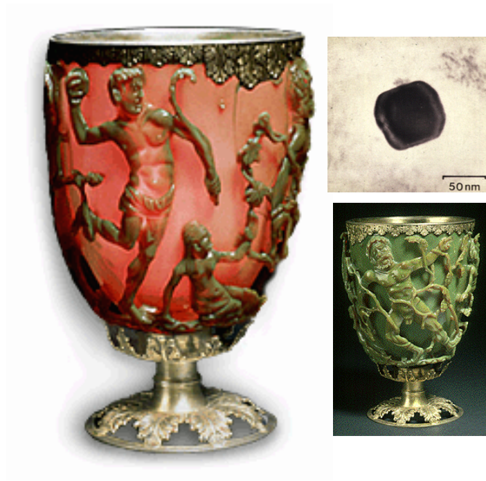
Figure 2. The Lycurgus Cup made from glass appears red in transmitted light and green in reflected light. The glass contains 70 nm particles as seen in the transmission electron micrograph. The cup itself is dated to 4th century AD, but the metallic holder is a later addition. From the site, http://www.thebritishmuseum.ac.uk .
