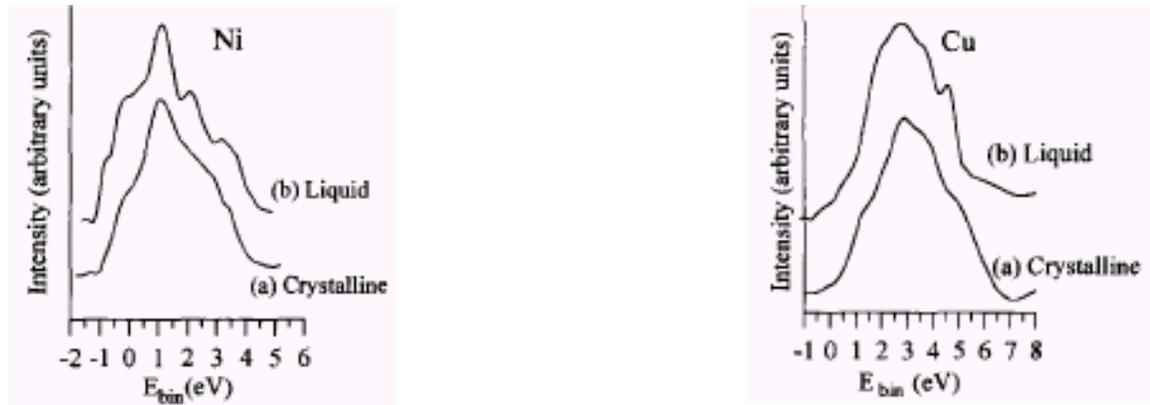
**Fig: 14** The XPS spectra of the valence band of (LHS) Ni: (a) crystalline state at room temp; (b) liquid state at 1850 K and (RHS) Cu: (a) crystalline state at room temperature; (b) liquid state at 1700K.<sup>[3]</sup>
