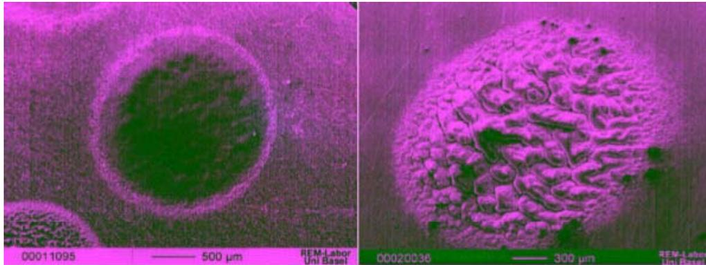
**Fig: 10** LHS: SEM picture <sup>[4]</sup> of laser treated niobium (~90 000 melting cycles). The flat irradiated area is clearly visible.
