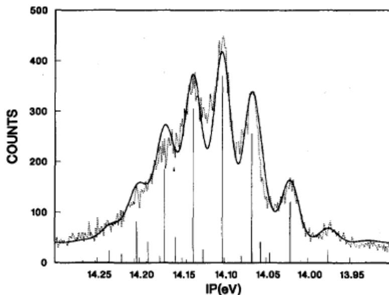
This is the comparison of a frank-Condon factor calculation With the  $C^2\Sigma_g^+$  state experimental spectrum of  $ZnCl_2^+$ . The individual lines are the calculated Frank-Condon Factors, each of which is convoluted with a Gaussian (0.024 eV width) to compare to the experimental spectrum (- calculated, .... Experimental)
