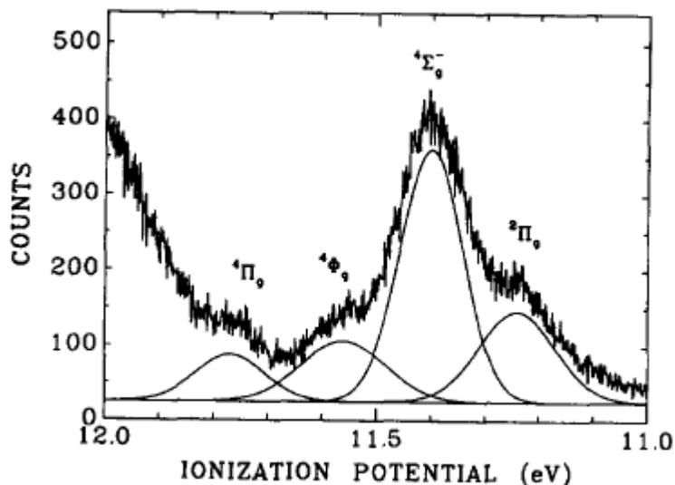
Here only four components are evident, by either visual inspection or curve fitting. Additional peaks may be present either coincident in energy or with low intensity. Some intensity is observed in ionization from each of the d orbitals,  $9\sigma_g$ ,  $3\pi_g$ , and  $1\delta_g$ .
