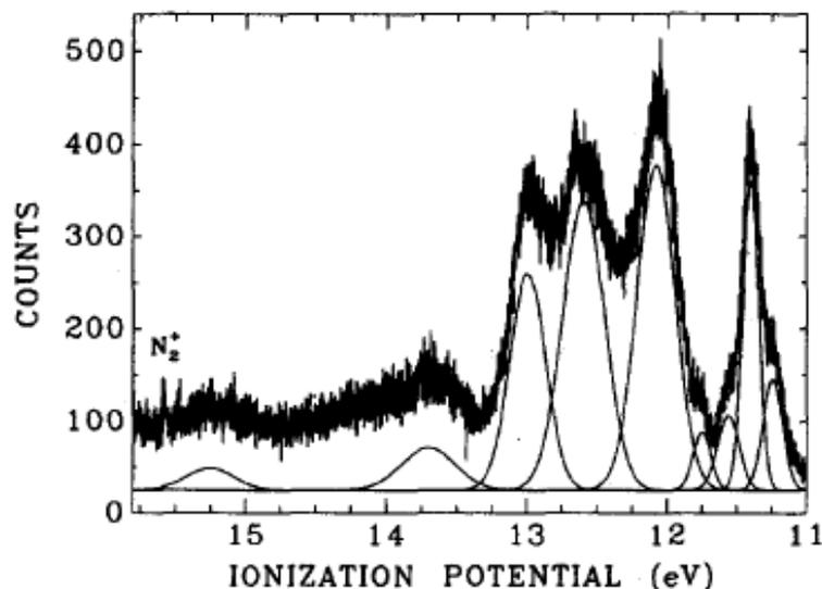
There are mainly four bands observed in the spectra which are from the d orbitals, on the basis of their small band widths. Some nitrogen impurity from the background at high ionization energy is observed. The rest of the spectrum can be assigned by analogous with those of  $\text{ZnCl}_2$  and  $\text{MnCl}_2$  as shown in the following table.
