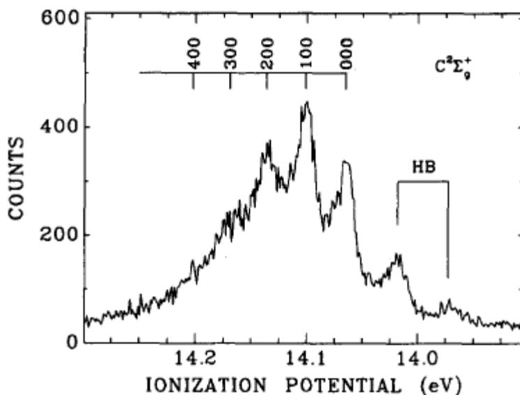
The He I photoelectron spectrum from the  $9\sigma_g$  orbital of  $\text{ZnCl}_2$  with the vibrational assignments. The vibrational levels are labeled with the  $\nu_1$ ,  $\nu_2$  and  $\nu_3$  vibrational quantum numbers. HB stands for the hot band transitions.
