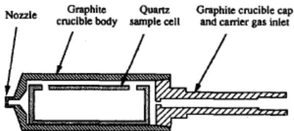
Here shown is the graphite crucible configuration with a sample cell.
