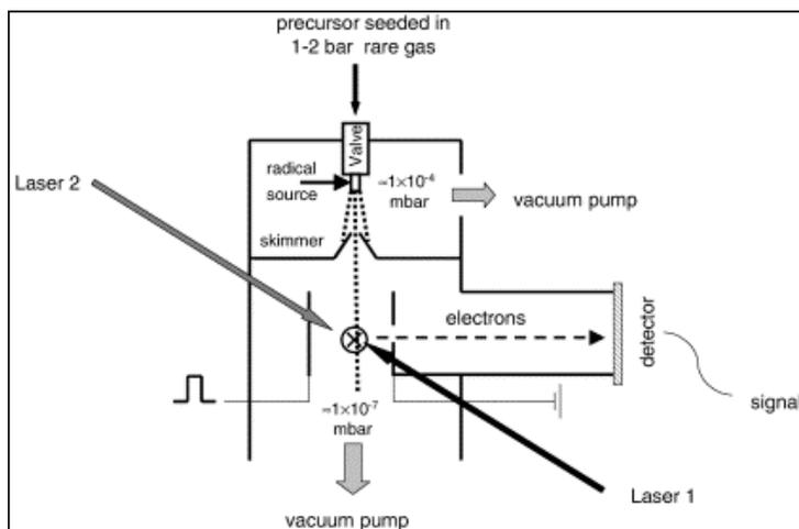
**Figure 3-** The schematic representation of the experimental setup.
