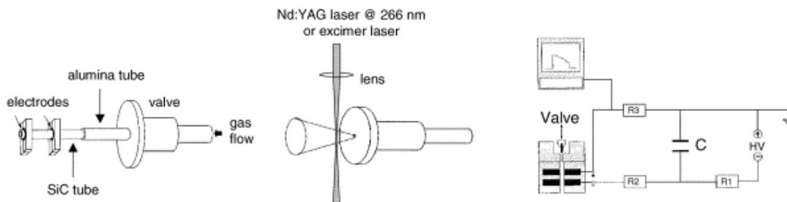
**Figure 1-** the schematic diagram for Flash photolysis, Pyrolysis, and electric discharge.
