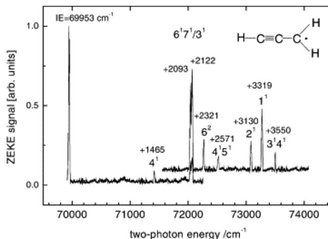
**Figure 7-** The ZEKE –spectrum of propargyl radical.
