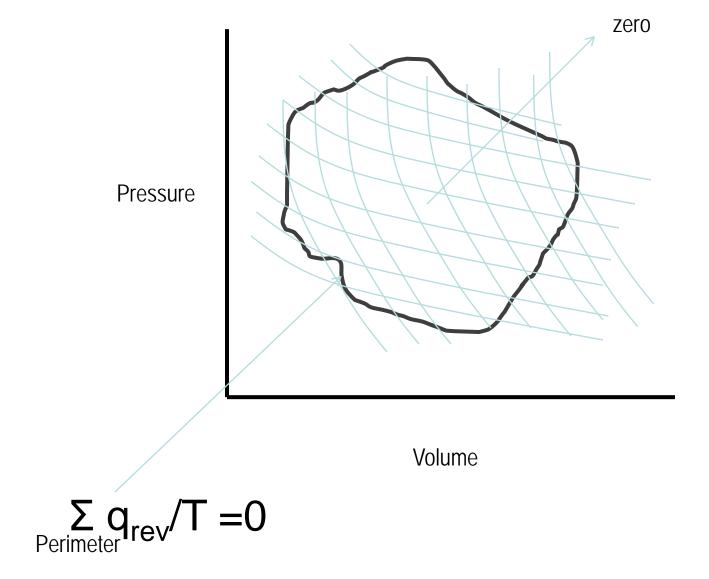
The Carnot cycle gives the maximum work that can be produced from an engine working between two temperatures. The work required in the refrigerator is the minimum work necessary to transfer heat  $q_c$  forms the reservoir at  $T_c$  to a reservoir at  $T_h$ .
