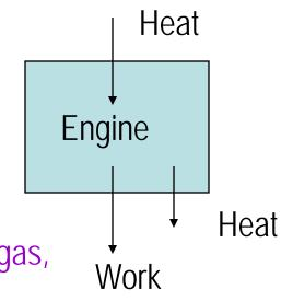
At the end of expansion, the system is not capable of doing work. To do work, it has to be brought back to the original condition by an **adiabatic step**. Thus a **cyclic process** is involved.
