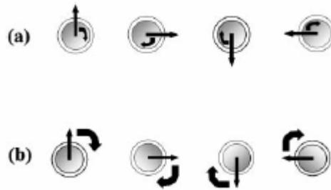
**Figure3.** (a) Neel rotation of magnetization in a magnetic particle (the particle does not rotate). (b). Brown rotation (the particle as a whole rotates).[2]
