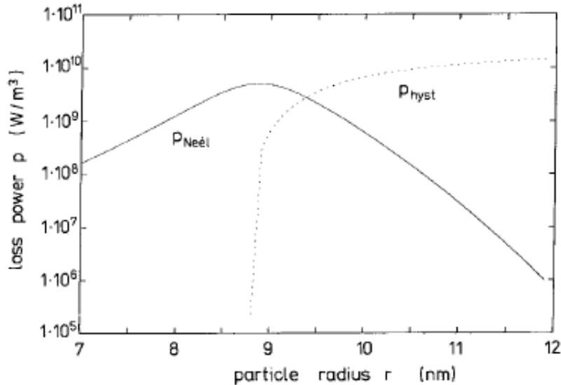
**Figure 4.** Dependence of magnetic loss power density on particle size for magnetite fine particles (dotted line—hysteresis losses, full line— Nèel losses; frequency  $2 \times 10^6 \text{ s}^{-1}$ ; field amplitude 6.5 kA/m) [2]
