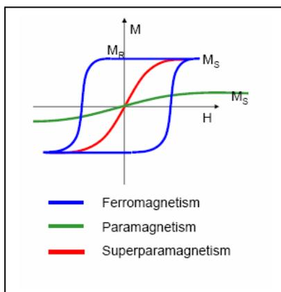
**Figure2.** Graph showing the differences in the M vs H curves for ferro, para and supermagnetic materials.
