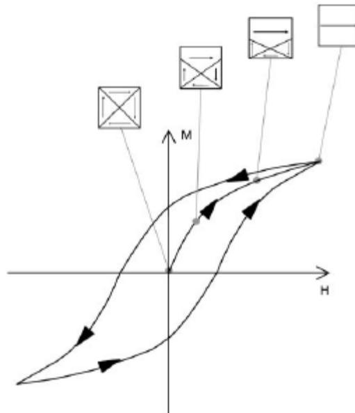
**Figure1.** Hysteresis cycle of a multidomain magnetic material (H is the magnetic field amplitude, M is the magnetization of the material) and domain wall displacements in such a material. The arrows indicate the direction of magnetization in the respective domain.[2]
