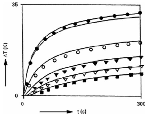
**Figure 11.** Temperature increase  $\Delta T$  as function of time for different reduced distances  $r/R$  from the composite centre. The points are experimental points for similar values.[10]
