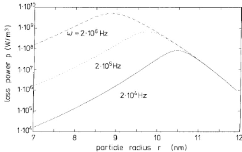
**Figure 5.** Grain size dependence of the loss power density due to Néel relaxation for small, ellipsoidal particles of magnetite (field amplitude 6.5 kA/m). ( $\omega = 2\pi f$ ) [2]
