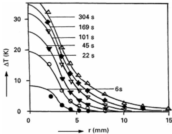
**Figure 12.** Temperature increase  $\Delta T$  as function of the distance from the composite centre for different exposure times. Measured values for the same parameters are plotted with symbols indicating the different exposure times. [10]
