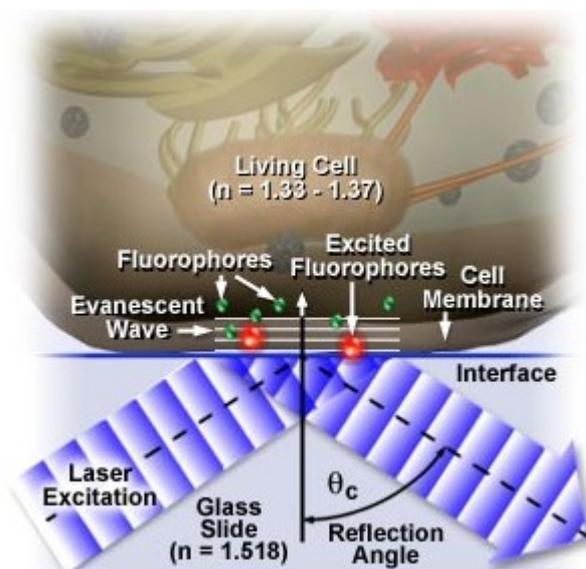
TIRFM, also called evanescent wave microscopy, selectively excites the fluorophores by impeding the beam at a high angle causing it to totally internally reflect (TIR). TIR generates a very thin electromagnetic field in the liquid
