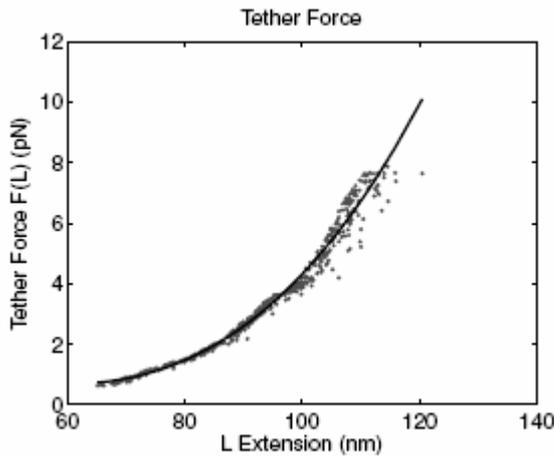
The solid curve is a cubic polynomial with coefficients fit by the method of least squares to the reconstructed force-extension profile of the tether.
