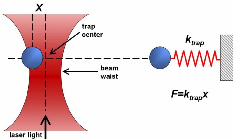
Fig 12: Diagram of optical trap showing its equivalence to a linear spring
